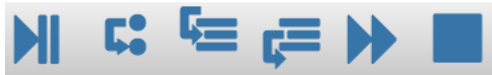
Figure 1: Spyder debug controls: Run/Pause, execute next line, step in, step out, run to breakpoint, stop
